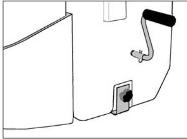
It is necessary to secure your toilet to the floor using the two L-brackets.
