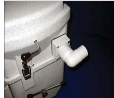
If a sharp 90 degree turn from the fan housing is needed, a 1¼ inch PVC street elbow (not provided) may be used to achieve a proper configuration.
